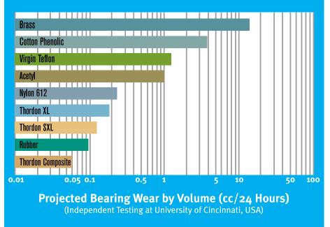
NOTE: Wet third particle abrasion. Shaft material: carbon steel, Bearing I.D.: 2.5cm (1 in.); Abrasive slurry mixture: 2% bentonite, 6% sand, 6% clay, 86% water.
